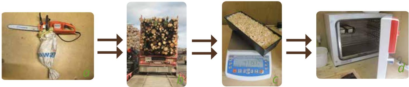
The quality needs to be assessed and measured at the BLTC. The **moisture content** is one of the most important quality measures. In the images you can see sampling of incoming raw material and moisture measurement according to the ISO standards:
